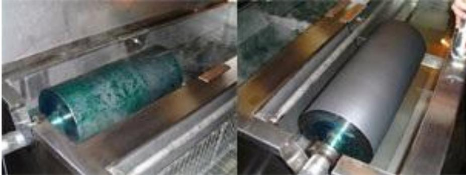
An Anilox Roller before and after ultrasonic cleaning
