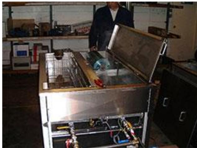
Above: an ultrasonic cleaning tank with in-line waste water recovery
